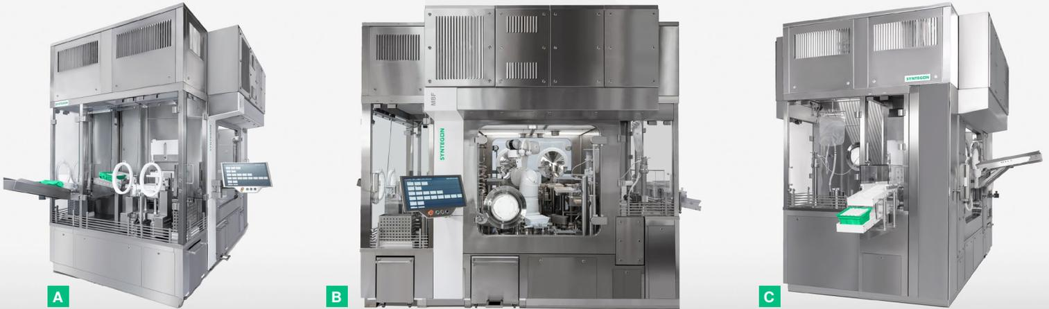
**What happens when two equal partners take on a new challenge? In the case of Vetter and Syntegon, the answer is “Versynta microBatch”. The fully automated, gloveless, Annex 1-compliant production cell for the aseptic filling of very small batches opens up new perspectives for both companies and underlines their respective pharmaceutical and technological innovative strength.**
