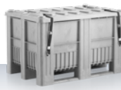
CB1 | 470 L 50H/X/.../F/CRAEMER BVT 40511/1800/500 ① 1200 x 800 x 740 mm ② 1236 x 836 x 766 mm Max. gross weight: 500 kg Standard colours: ■
