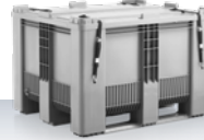
SB3 | 610 L 50H/X/.../F/CRAEMER BVT 40513/2160/600 ① 1200 x 1000 x 790 mm ② 1218 x 1018 x 834 mm Max. gross weight: 600 kg Standard colours: ■
