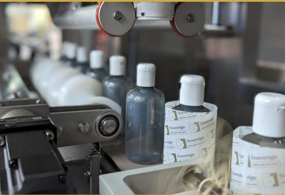
Our sleeving machines have been used worldwide in various industries for many different uses, including pharmaceutical, food and beverage, DIY, cosmetics and more. Sleeving offers a fantastic alternative to labelling, where self-adhesive labels are not suitable, with the added benefit of having 360-degree branding space on each product.
