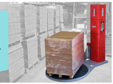
Machine rolls are manufactured in 500mm width rolls using either a cast film or nano film. The cast film rolls are available with 150% stretch for standard pallet wrappers or 250% stretch for power pre-stretch machines.
