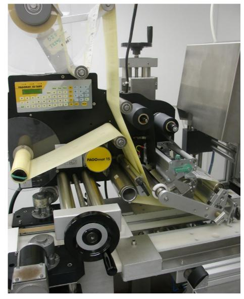
Verification with print quality inspection and ID/code reading the UDI can be checked in real time through the whole production cycle to confirm compliance to the FDA specifications. The UDI can be applied to labels, boxes, products, components and devices – therefore a generic approach to the quality
