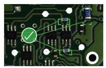
Inspect for incomplete or excess solder, missing components or misaligned/rotated parts.
