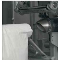
Spillage rejecting flap during bag discharge
