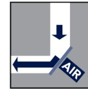
The pressure chamber aeration concept provides optimum product flow with minimal air consumption. Aeration rates depend on the product characteristics and are individually adjustable.
