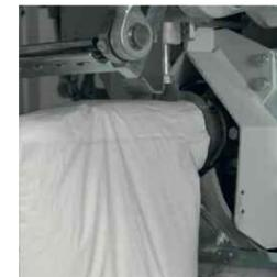
Spillage rejecting flap during filling process
