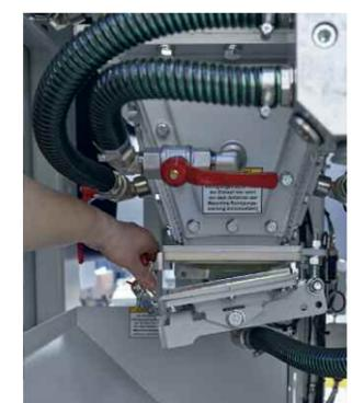
Maintenance flap at the filling box chamber
